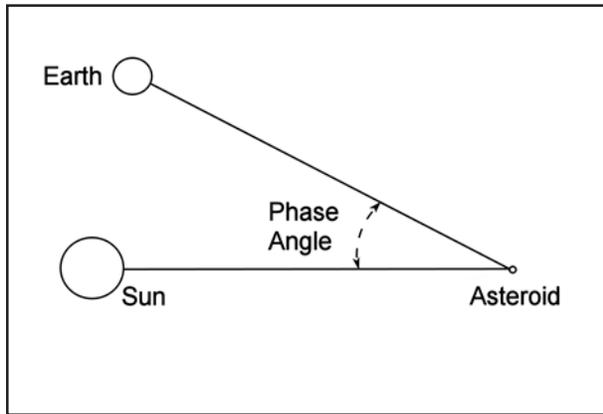
*Figure 1: The phase angle is that observed at the asteroid between the lines of sight of the Earth and Sun.*
