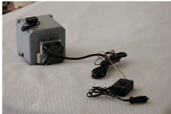
Cooler assembly with 12V connector and switch
