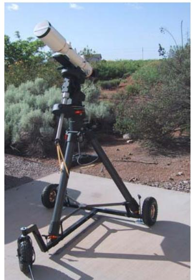
*Figure 3: Remote controlled driveway system*
