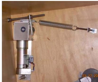
*Azimuth motor installed*
