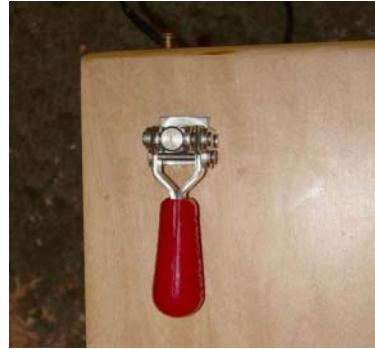
*Azimuth engage lever*
