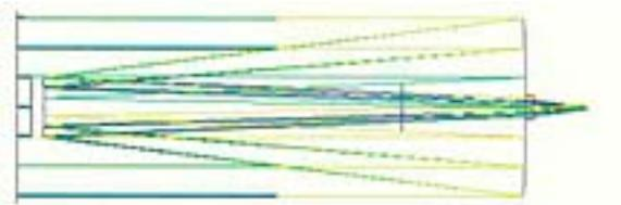
*Figure 3. F/10 Classical-Cassegrain telescope with focal reducer lens (small rectangle touching back surface of primary mirror).*
