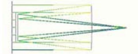
*Figure 2. F/4 Classical-Cassegrain telescope*
