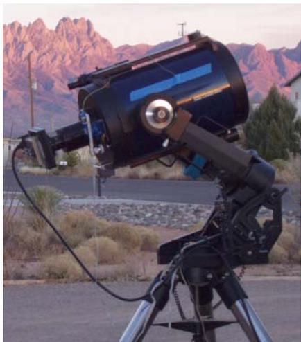
*The 12-inch LX-200 Classic with Apogee AP-7b camera and RoboFocus bolted down into its observing position. An umbilical runs back to the garage to allow the telescope to be controlled by the computer located there.*
