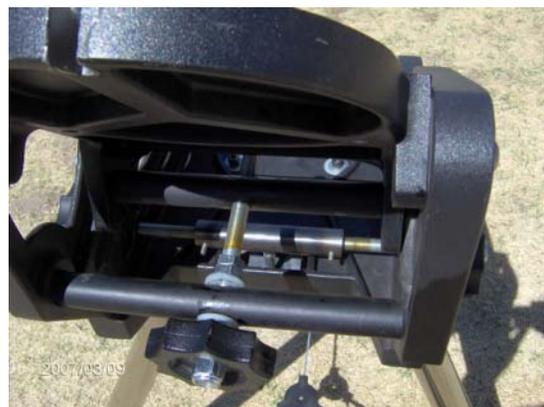
This follower yields an azimuth adjustment with very little slop. As you can see in this photo, it covers a much wider span of azimuth screw than the original, and exhibits almost no tilt when reversing directions.
