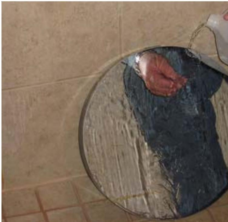
This is done with distilled water. I found that Walgreens has gallon jugs of distilled water for under \$2.00. Most of the water droplets should run off the mirror. However, it is important to not let water drops dry on the mirror surface.
