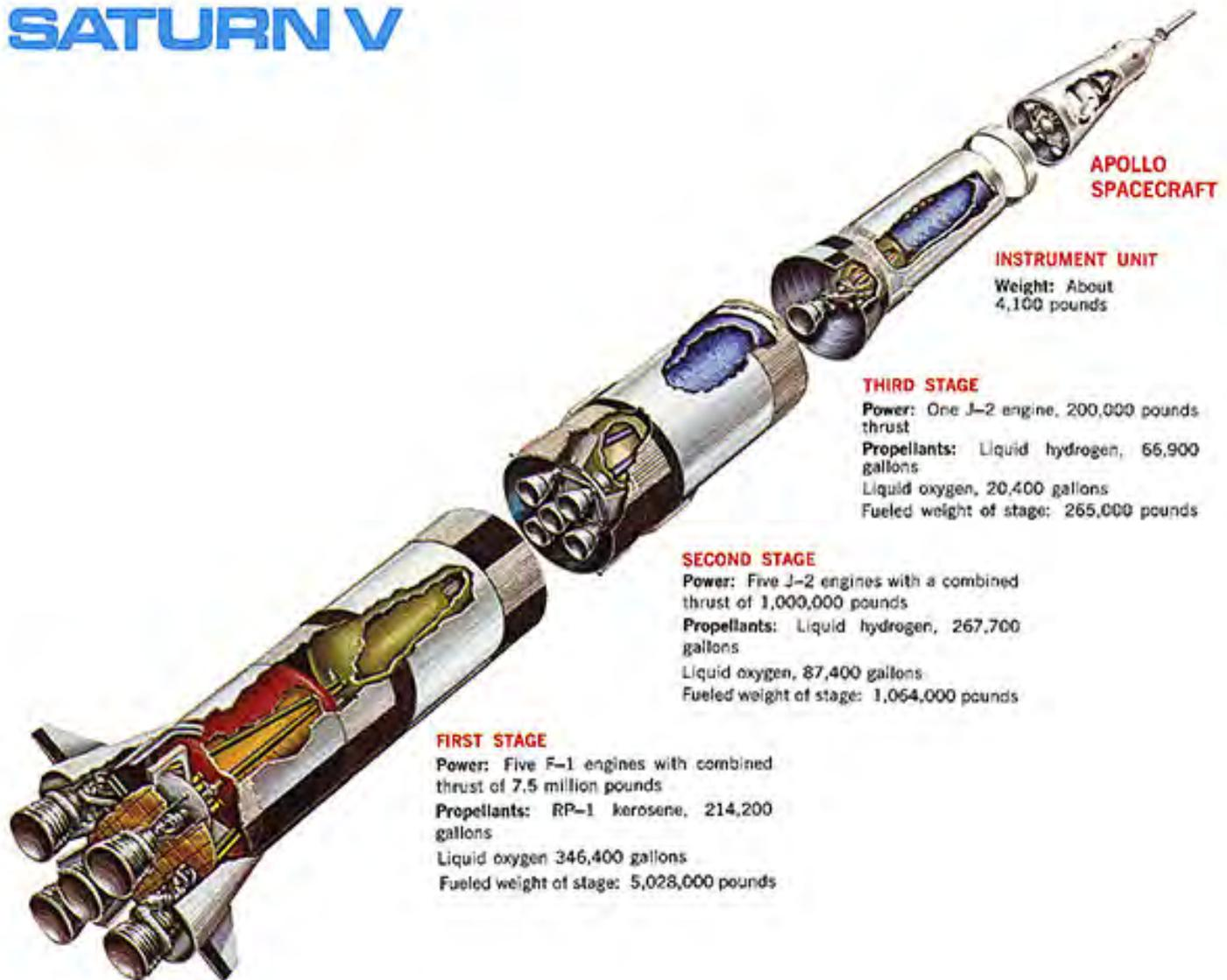
**Figure 2: Saturn V Cut-away.** A rocket like the Saturn V is divided into multiple stages. Each stage accelerated the payload to a higher speed before it is dropped to fall into the ocean. Only the top stage is traveling fast enough to make orbit.
