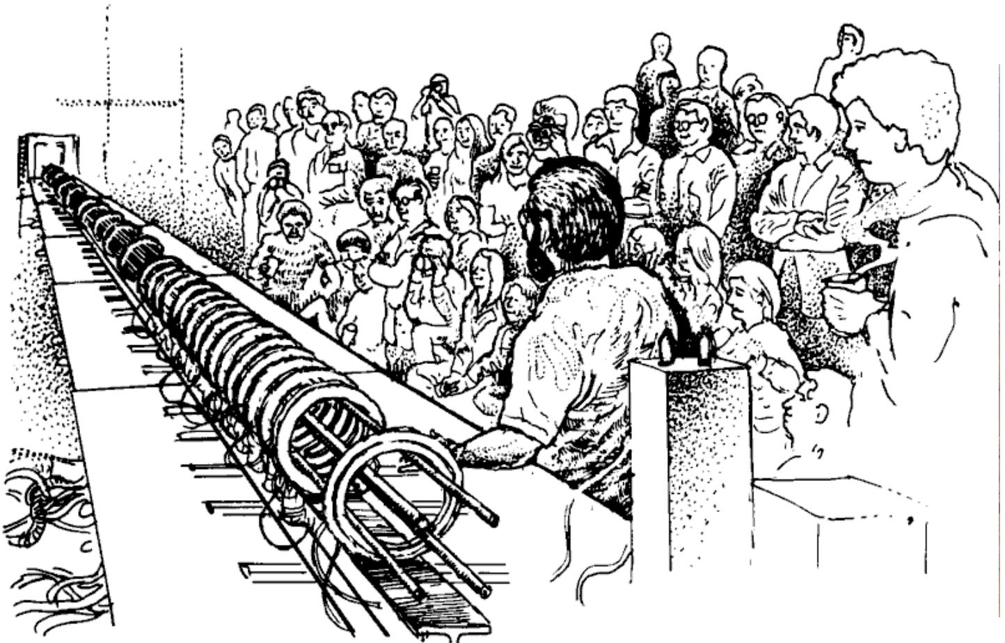
**Figure 3: Mass Driver Concept.** Don Davis's drawing of an experimental mass driver. The test mass is propelled down the track by the magnetic fields generated by the ring electromagnets. The electromagnets are controlled by a computer program that monitors the motion of the mass down the track and turns the electromagnets on and off as needed. Copyright Don Davis.
