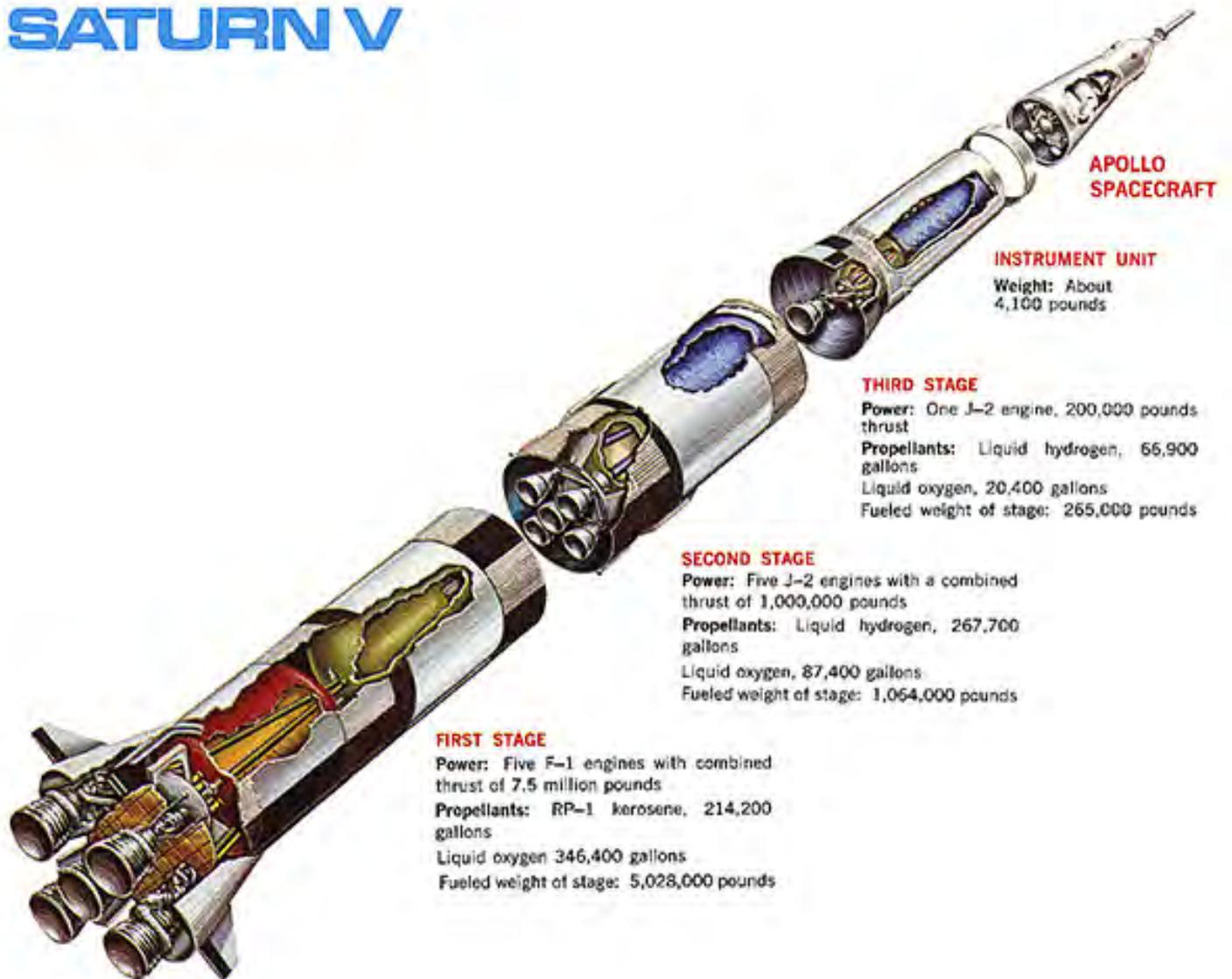
**Figure 2: Saturn V Cut-away.** A rocket like the Saturn V is divided into multiple stages. Each stage accelerated the payload to a higher speed before it is dropped to fall into the ocean. Only the top stage is traveling fast enough to make orbit.
