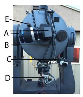
Rear view of parked telescope. A is the eyepiece and diagonal. The diagonal can be rotated to facilitate viewing depending on the scope position by loosening thumb screws on the side. B are the data cables that run around the scope and through the mount. THESE ARE THE CABLES YOU NEED TO MONITOR CAREFULLY DURING TELESCOPE SLEWING (i.e. moving to different areas of the sky) C is the finder scope. D is the Mallincam video camera. E is the main focuser for the 16
